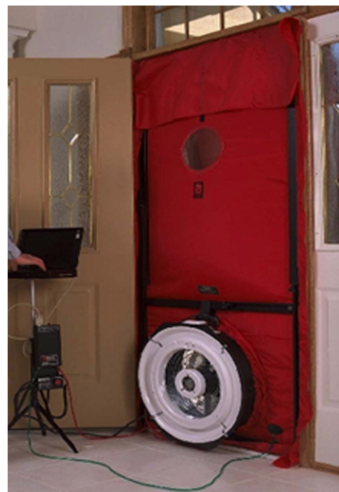
Fig. 7. Blower door method to measure air tightness performance.
